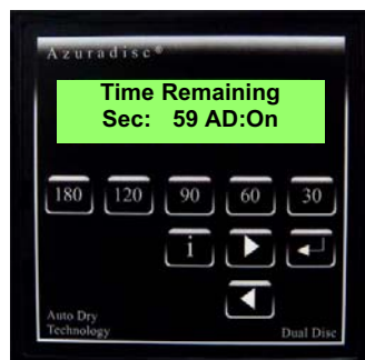
Number = Length of time in seconds After pressing selected amount the screen will show time remaining
