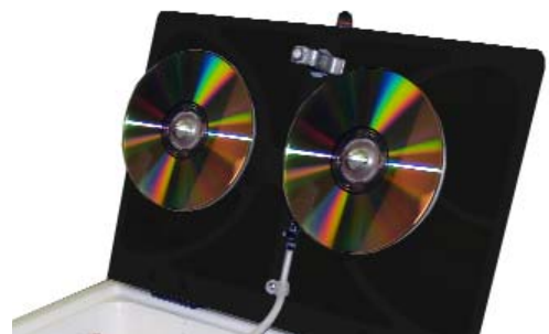
After repair cycle is finished remove CD's or DVD's from spindles.
