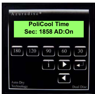
Number = Length of time in seconds After pressing selected amount the screen will show time remaining
