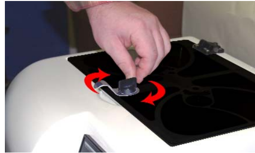
Close the lid, press and turn latch clockwise until it moves passed resistance.
