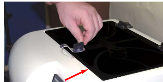
For the lid to be sealed the edge must be flush with the interior bevel of the cabinet as shown above.
